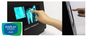
JDI's in-cell hovering technology enables touchless input/output of information and robust visibility.
