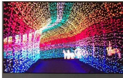
Newly developed polarized laser backlight LCD
