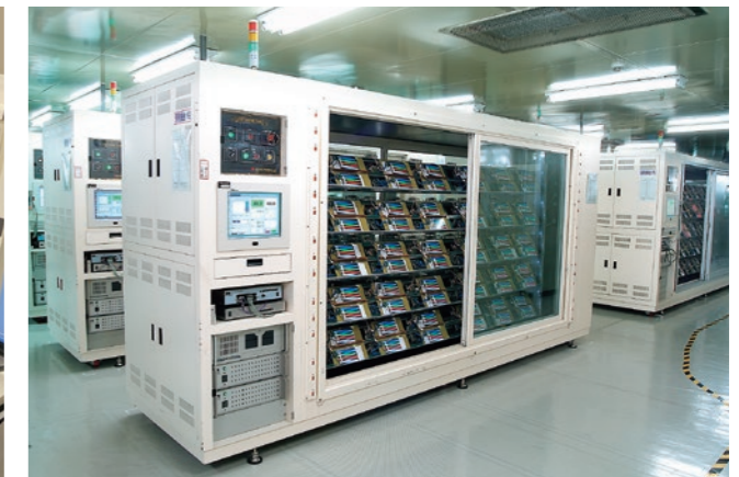
Aging inspection during the manufacturing process
